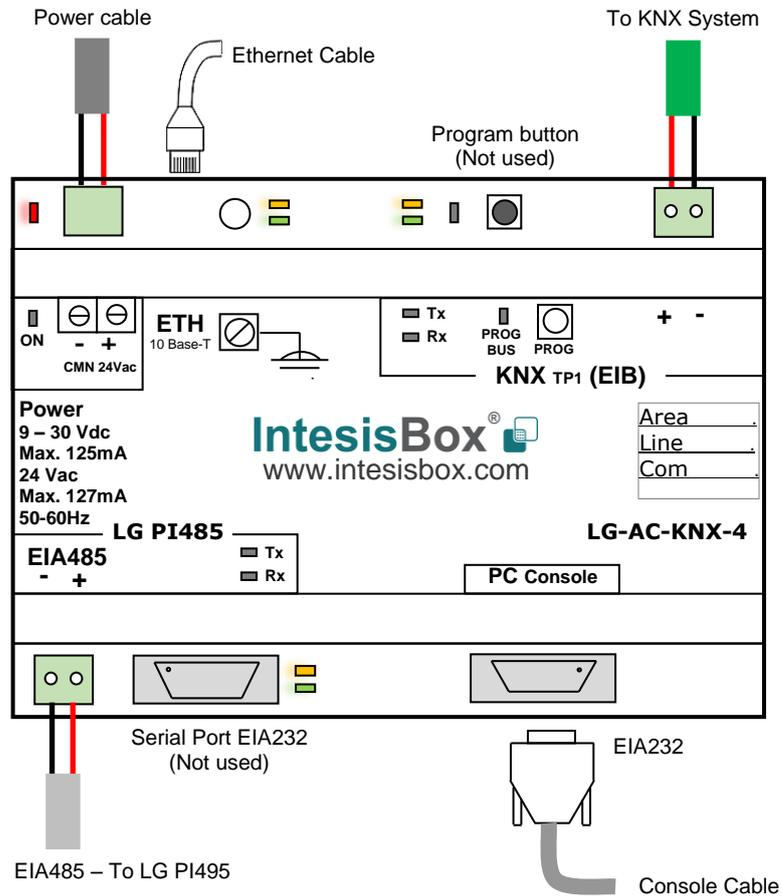
**Figure 2.1** IntesisBox® LG-AC-KNX connection diagram
