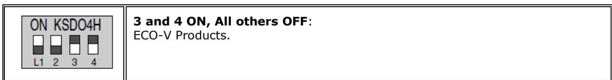
**Figure 8.5** **Figure 8.6** **DIP Switch configuration**
