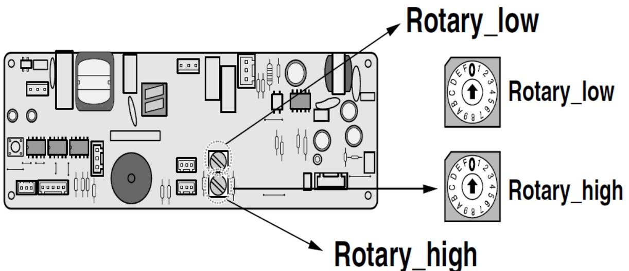
**Figure 8.7** DIP Switch configuration
