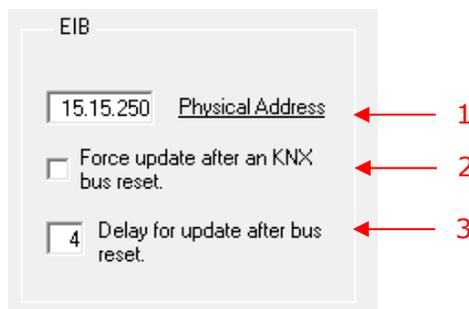
Figure 3.3 KNX interface configuration’s parameters.
