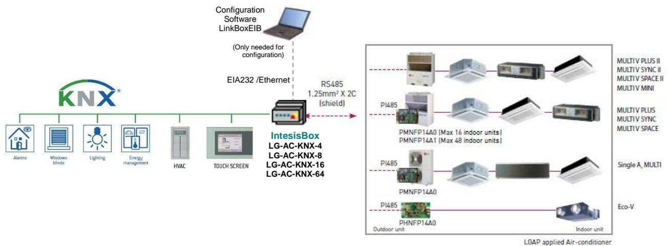
**Figure 1.1** System integration using IntesisBox® LG-AC-KNX.
