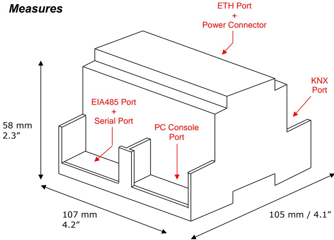
Recommended available space for its installation (to keep proper space among all connectors when these ones are installed):
