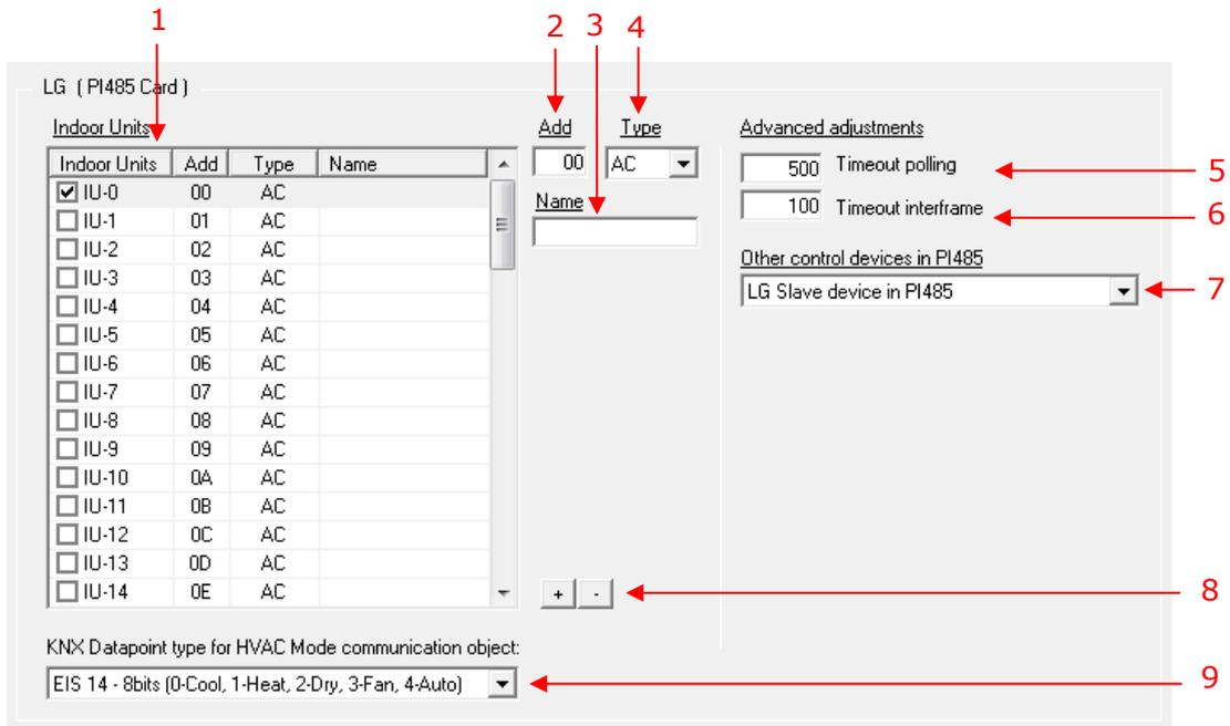
**Figure 3.6** Parameters for LG'S AC System (PCB PI485)
